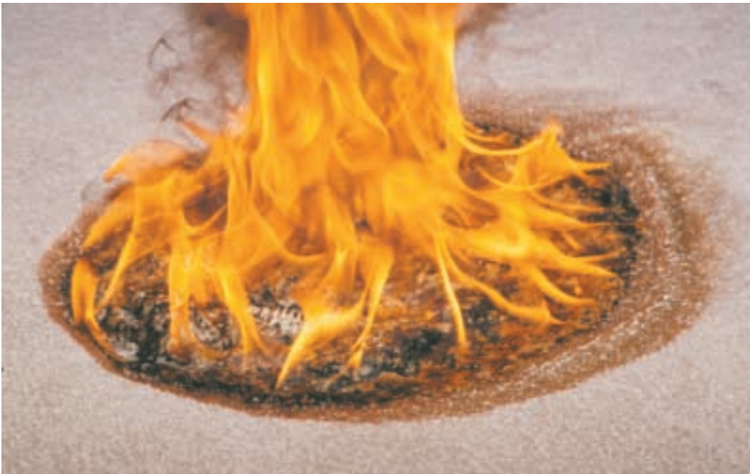
Figure 20. Closeup view of 250 mL gasoline fire on carpet 2
