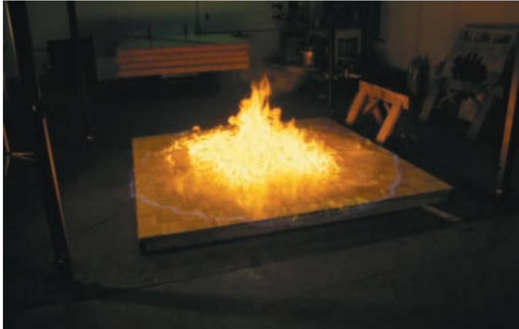
Figure 5. Ignition of 1,000 mL gasoline spill on wood parquet flooring
