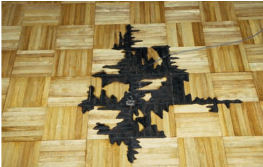
Figure 14. 1,000 mL kerosene spill burn pattern
