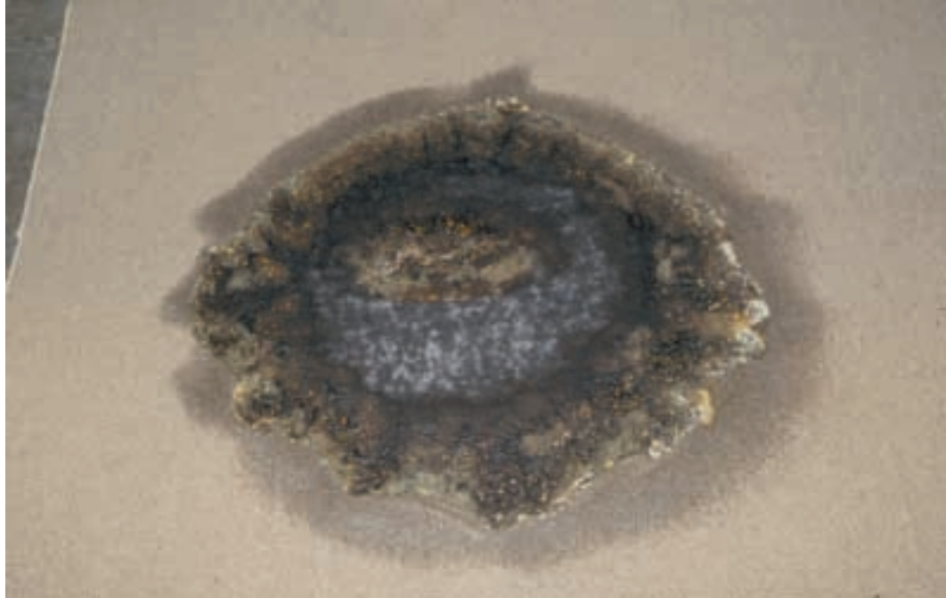
Figure 21. Doughnut burn pattern on carpet 1. 250 mL gasoline fire extinguished at approximately 146 s with CO 2 .
