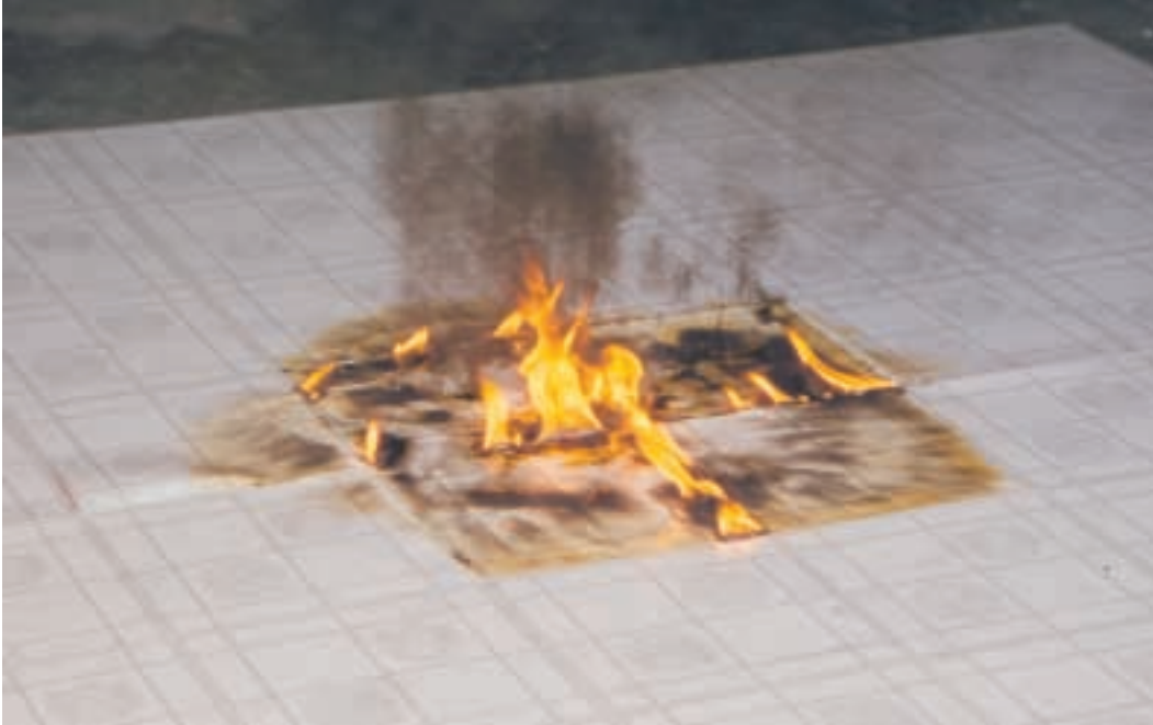
Figure 7. Burning in the seams of the vinyl tile flooring
