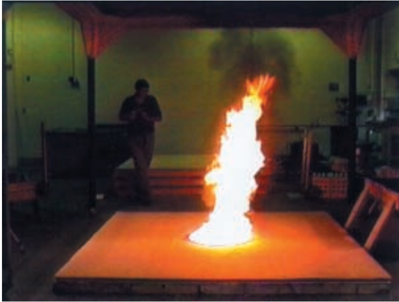
Figure 15. 1,000 mL gasoline spill fire on carpet 1 at approximately 10 s
