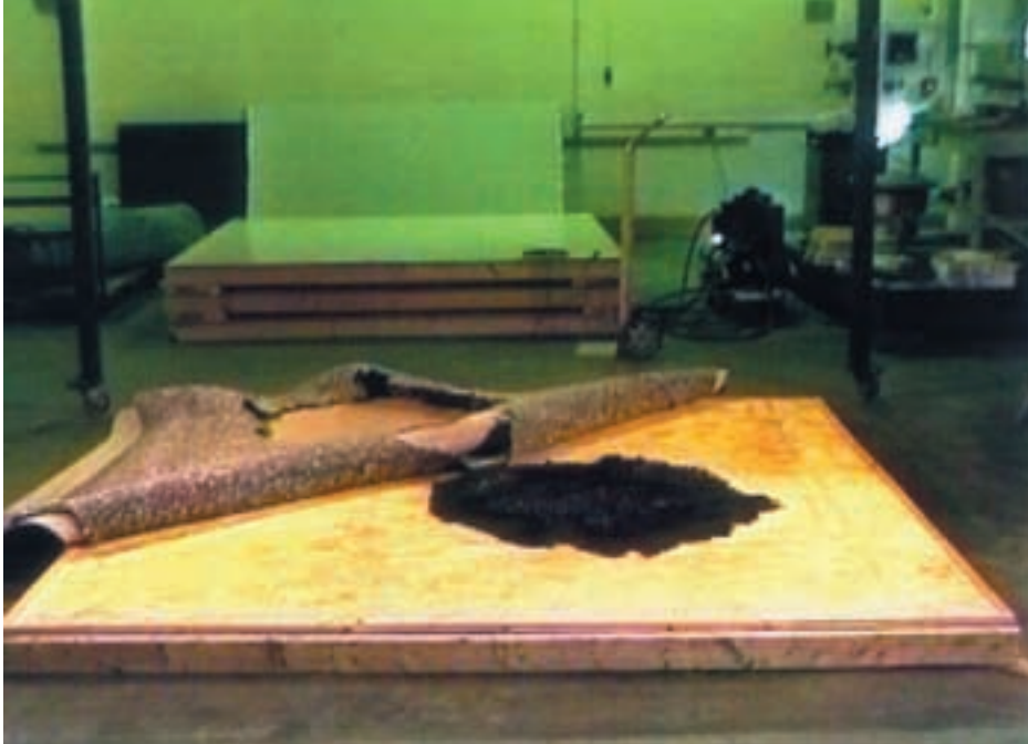
Figure 27. Carpet and padding removed from floor leaving doughnut pattern behind. Results shown for 250 mL gasoline spill on carpet 1 extinguished with CO 2 after approximately 213 s of burning.
