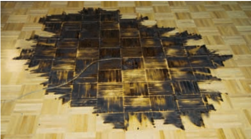
Figure 8. 1,000 mL gasoline spill fire burn pattern on wood parquet floor
